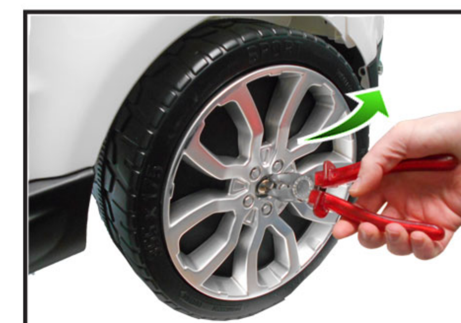
2. Remove the aranlock and the washer.
