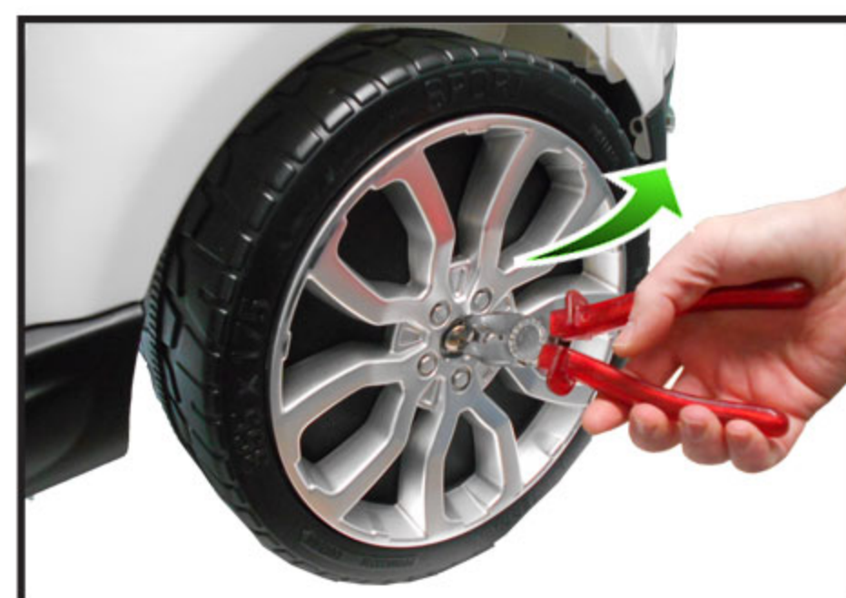
2. Remove the aranlock and the washer.
