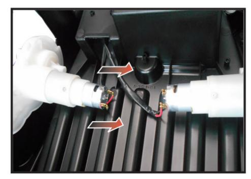
7. Disconnect the wires of the mechanism t.
