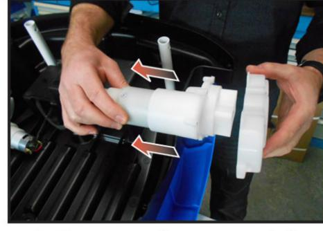
8. Separate the cover of the mechanism to replace it with a new one. Re-assemble in reverse order.
