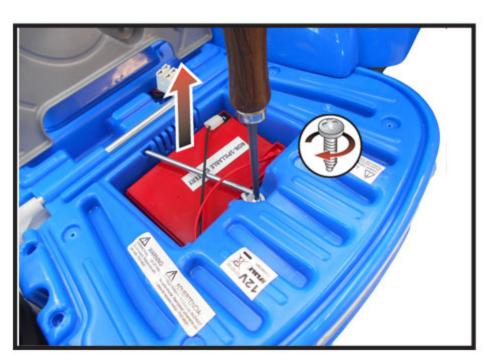
2. Unscrew the axle to remove the battery.
