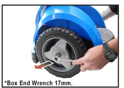
1. Unscrew the nut whilst holding the nut on the other side, to remove it.
