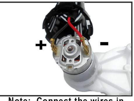
Note: Connect the wires in same polarity order of the previous mechanism.
