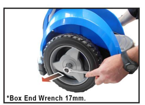
1. Unscrew the nut whilst holding the nut on the other side, to remove it.
