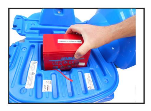
4. Remove the battery and replace with a new one. Re-assemble in reverse order and pay attention to connecting the wires to the proper polarity.
