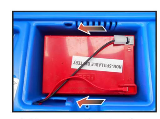
3. Disconnect the wires from the battery.
